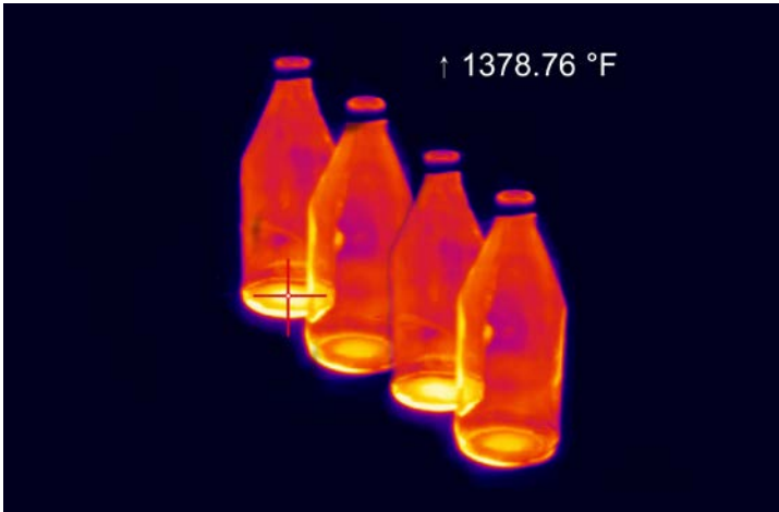
Hot spot detection at glass bottle production
