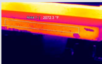
Run-off area of a continuous casting plant
