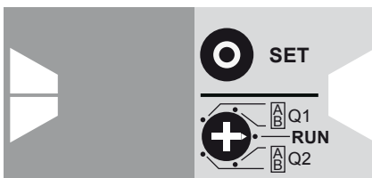
ILR103x: Adjust analog output and switching output via touch keys
