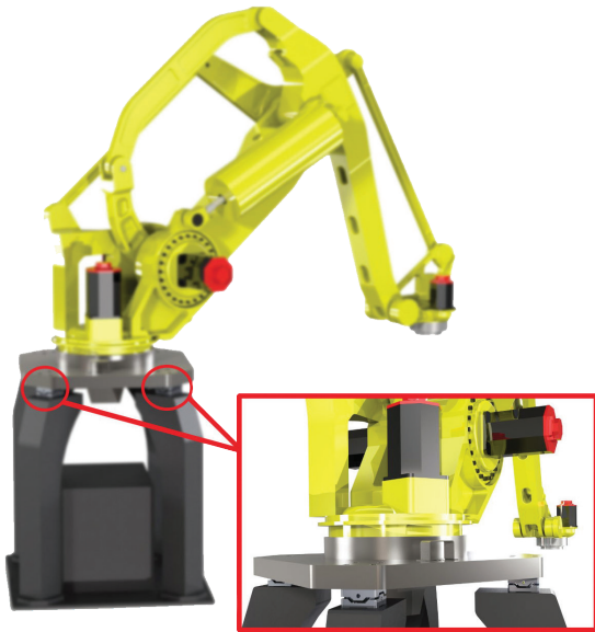
Load Cells are commonly used in industrial applications to measure forces and moments.
