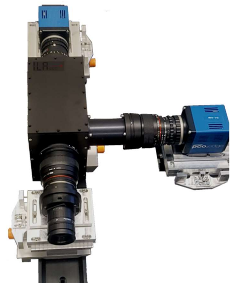
Fig.3: DGV camera module with an iodine filter
