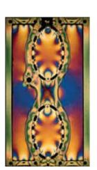
PhotoStress stress patterns of an aircraft fuel door panel under load
