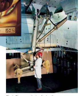
PhotoStress analysis of a landing gear
