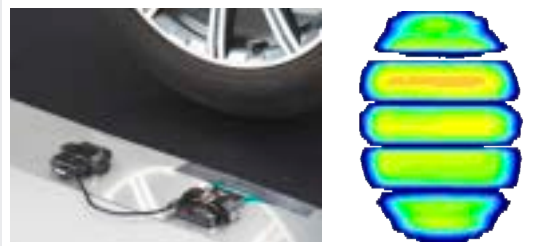
Shows contact shape and pressure distribution of fast moving tires
