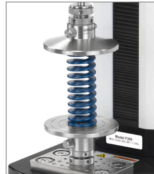
Compression spring testing
