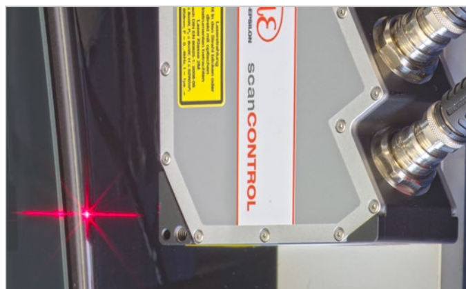
Gap measurement on car bodies
