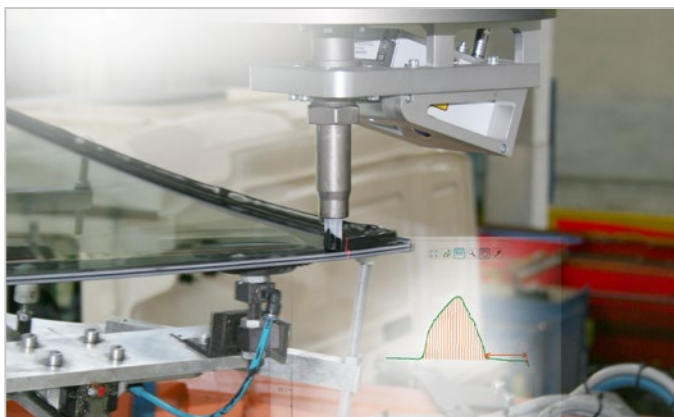
Inspection of the adhesive beading
