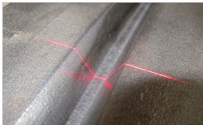
V-seam measurement on pipes
