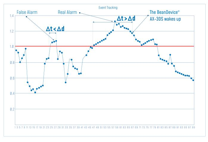
$\begin{array}{l} \Delta d : \text{shock detection hysteresis.} \\ \Delta t : \text{Observed duration} \\ \text{If } \Delta t = \Delta d, \text{ the shock event is detected and} \\ \text{recognized, the BeanDevice} \\ \text{wakes up and start data sampling} \\ \text{in "streaming mode".} \end{array}$
