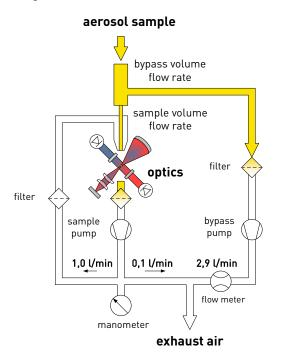
Schematic description of the operating principle of the LAP 323.
