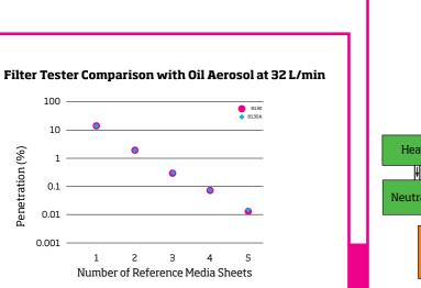
As shown in this example, the two tester models agree very well for  $% \left[ {{\left[ {{{\rm{AS}}} \right]}_{\rm{AS}}} \right]_{\rm{AS}}} \right]$ penetration testing of flat sheet media. An increasing number of sheets is used to cover a wide range of measured penetrations.
