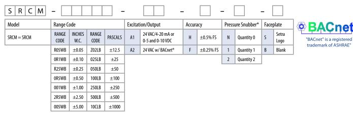
$Ordering\ Example: Part\ No.\ SRCMR05WBA1HNS\ for\ A\ SRCM,\ \pm0.05''WC\ Range,\ 24VAC/4-20\ mA,\ 0.5\%\ Full\ Scale\ Accuracy,\ No\ Pressure\ Snubber$
