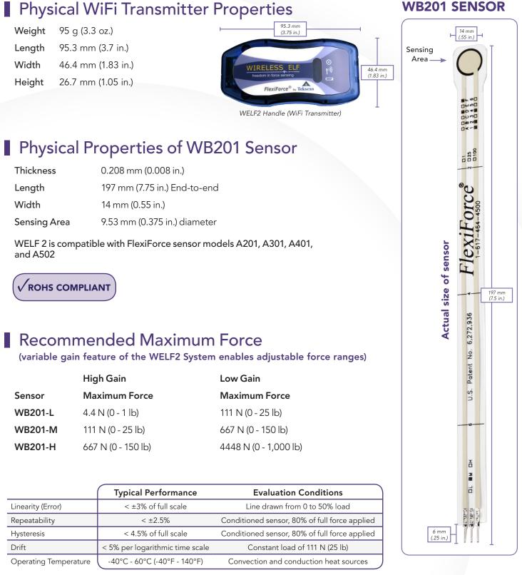
Force reading change per degree of temperature change = 0.36%/°C (±0.2%/°F)
