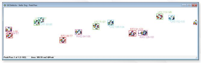
Software display of multiple paw strikes. Automatic strike detection determines where the paws have made contact with the Strideway.
