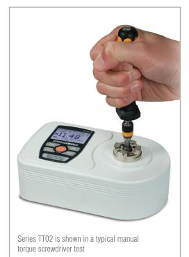
Series TT02 Torque Tool Testers present a simple and accurate solution for testing manual, electric, and pneumatic torque screwdrivers, wrenches, and other tools. These testers are compact and rugged, suitable for production environments. A universal 3/8" square receptacle accepts common bits and attachments. The TT02 captures peak torque in both measurement directions, and also calculates 1st and 2nd peaks, useful for click-type tools.
