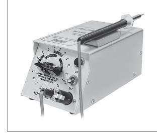
A time-proven precision soldering instrument for miniature and/or delicate soldering applications. Full 25-watt rating in 17 selector positions to handle all *M-LINE* solder alloys except 1240-FPA. Magnetic solder pencil holder and flexible, burn-resistant cord. Lightweight soldering pencil [1.1oz (31g)]. Specify 115 or 220 Vac, 50 or 60 Hz operation.
