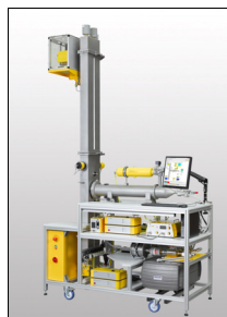
Filter test rig AFC 133 per as ISO 11057, VDI 3926 Part 1, version 1
