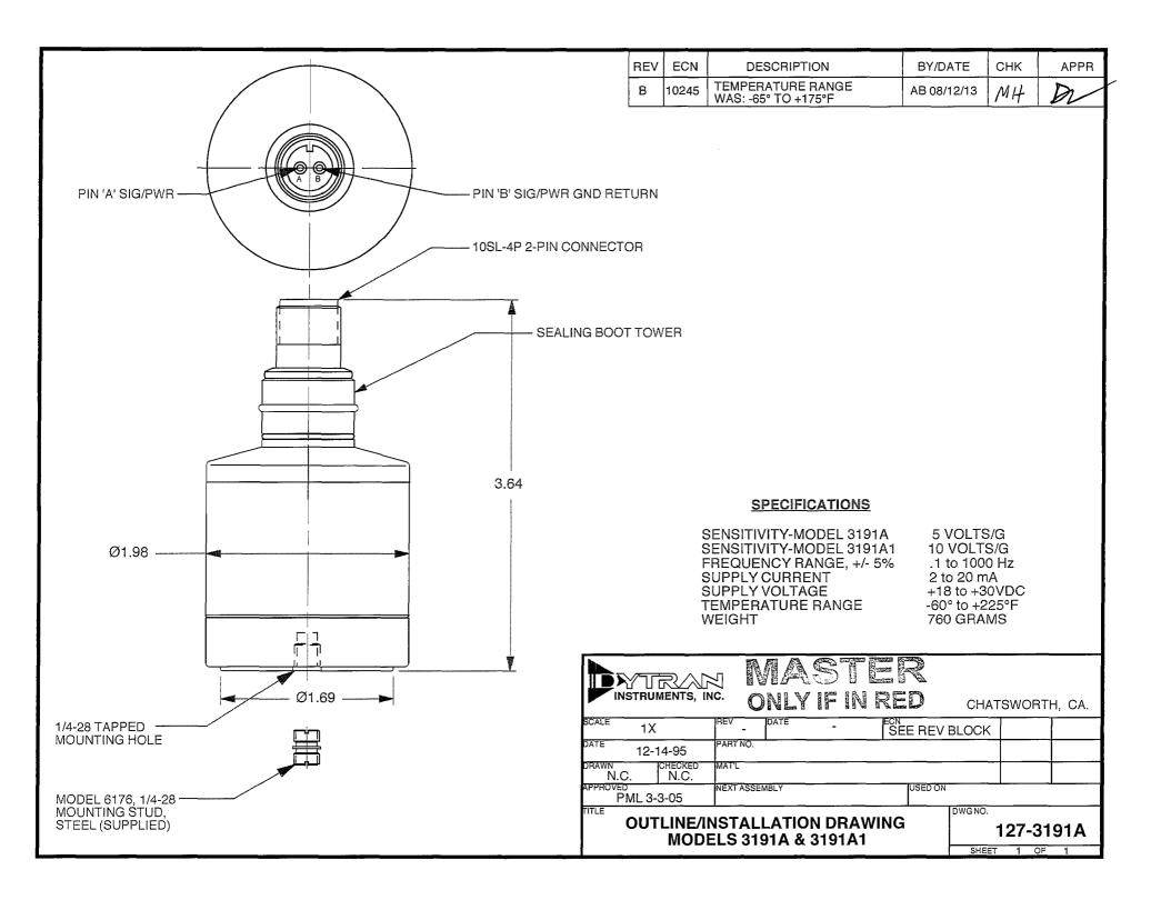
Model Number DOC NO PERFORMANCE SPECIFICATIONS PS3191A 3191A IEPE SINGLE AXIS ACCELEROMETER REV C, ECN 10367, 09/11/13
