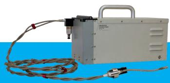
The TSI Nanoparticle Emission Tester (NPET) Model 3795 is a portable, accurate instrument capable of measuring total solid particle number emissions from a variety of diesel-powered sources, including construction machinery, buses, stationary gensets, and more. Featuring a robust, user-friendly design, the NPET can be used in the field by researchers, regulatory inspectors, and maintenance personnel alike.
