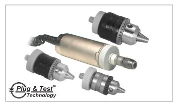
Series R51 smart sensors measure bi-directional torque for numerous applications across virtually all industries. Interchangeable Jacobs chucks and bit holder add flexibility for a variety of applications. The sensors can be used as hand held devices or mounted to a test stand. Superb overload protection adds peace of mind. Capacities available from 10 ozFin to 100 lbFin [7 to 1150 Ncm]. Compatible with Mark-10 indicators (sold separately) through unique Plug & Test<sup>TM</sup> technology.
