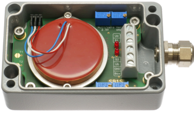
Sensorbox containing one sensor, one signal conditioner with 0.5 ... 4.5 Volt output and two open-collector output switches
