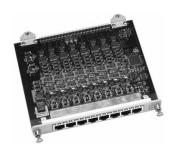
The Model 7003-8-HL High Level Input Card is used in conjunction with the Model 7003-8-A-I Analog Input Card to perform signal conditioning and excitation for high level (±10V) inputs.
