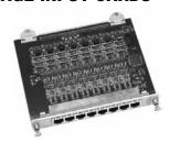
A choice of two Strain Gage Input Cards (7003-8-SG or 7003-8-SG-A) are used in conjunction with the Model 7003-8-A-I Analog Input Card to perform bridge excitation, bridge completion, shunt calibration, and signal conditioning for eight quarter, half, and full bridges. Note that the 7003-8-SG-A Strain Gage Input Card with Analog Output has an analog output which provides an amplified representation of the input source.
