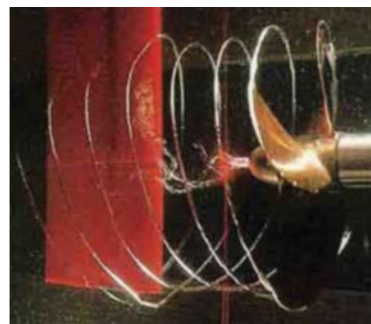
3D LDV System for the measurement of flow behind propeller, INSEAN, Italy
