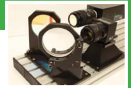
PLIF System using dichroic color separation arrangement for measuring velocity and scalar quantity
