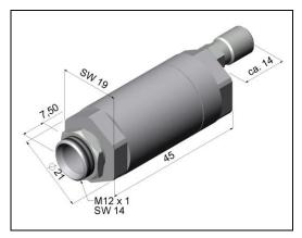
Standard air purge collar [ACCTAP] for optics with a D:S ≥ 10:1 (not for sensing heads with 32 mm length), fits to the mounting bracket Hose connection: 3x5 mm Thread (fitting): M5
