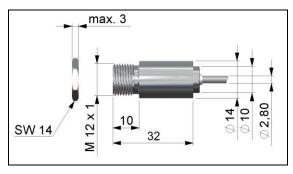
Sensing head LT15CF/ LT22CF/ 3MCF/ CTP7CF
