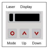
Pressing the Mode button again recalls the last called function on the display. The signal processing features **Peak hold** and **Valley hold** cannot be selected simultaneously.
