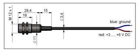
**OEM-Laser-Sighting tool [ACCTOEMLST or ACCTOEMLSTCB8]**
