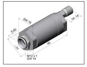
Standard air purge collar [ACCTAP2] for optics with a D:S ≤ 2:1 (not for sensing heads with 32 mm length), fits to the mounting bracket Hose connection: 3x5 mm Thread (fitting): M5
