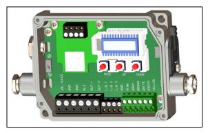
**Opened 4M electronic box with terminal connections**
