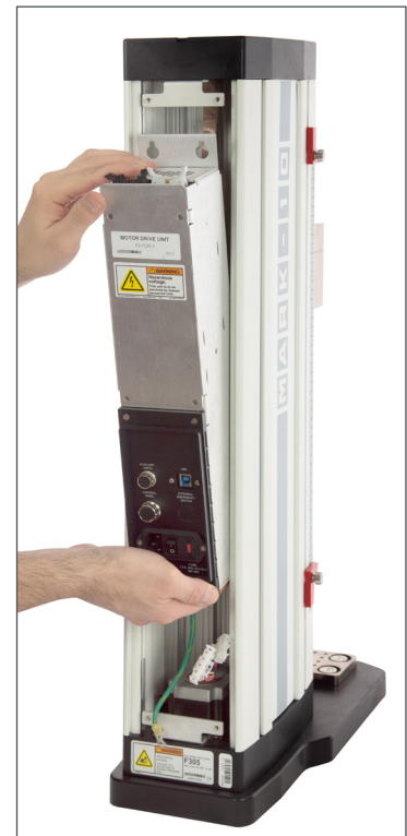
Removing the electronics module
