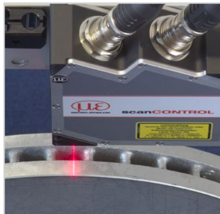
Profile measurement of the brake disc
