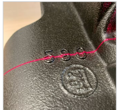
Text recognition on the cast part
