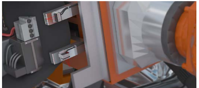
Fast position monitoring at the assembly robot
