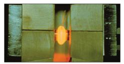
Strain Induced Crack Opening (SICO) Procedure: The SICO procedure is a quick and cost-effective method for thermomechanical process optimization in forging and forming operations.
