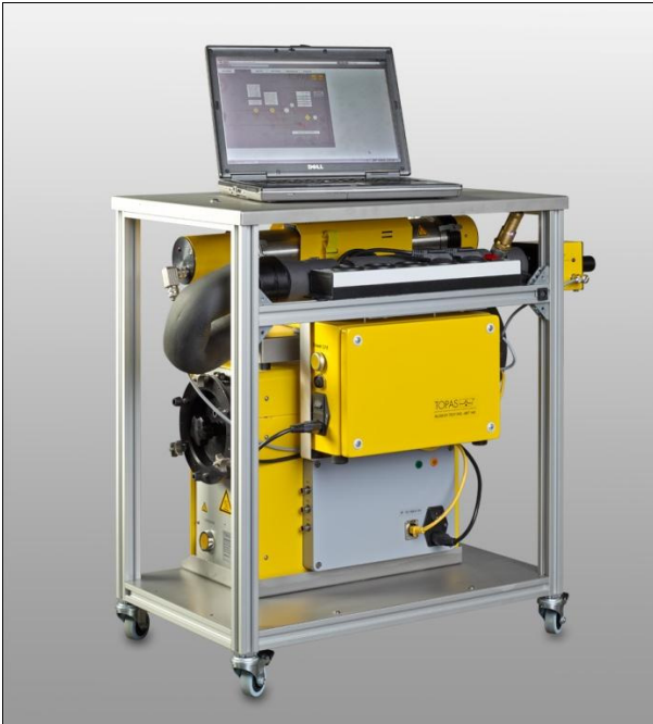
Blow-By Test Rig BBT 143 for measuring the oil concentration of blow-by gases: Gravimetric Measuring System GMS 141, Process Aerosol Photometer PAP 610 and PAP 612
