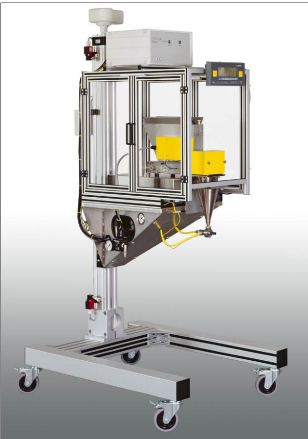
Dust Disperser SAG 420 on a weigh scale with housing
