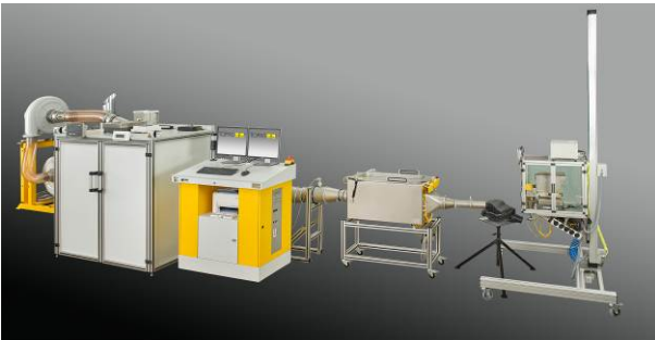
Automated dust test rig ABP 115 with SAG 420
