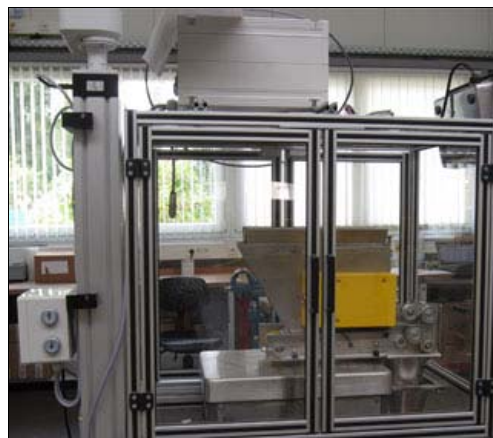
Dust Dispenser SAG 420 on a weigh scale
