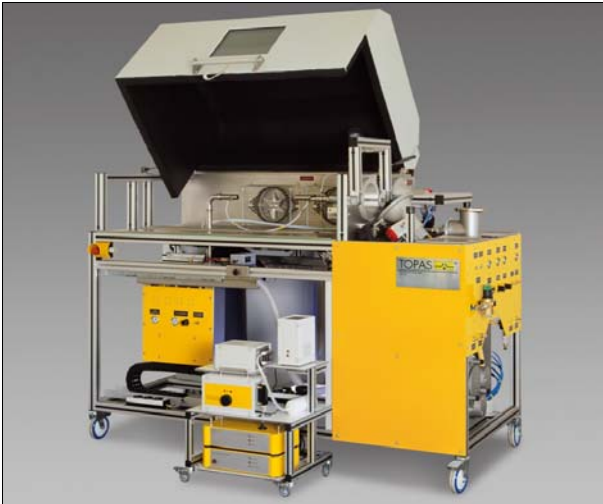
Separator Performance Tester SPT 140 Filter Test Rig for oil mist separators
