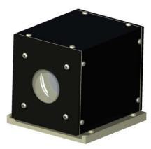
Fig. 5: Vapor cell heater
